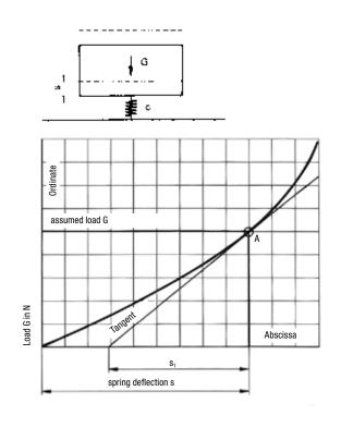
The determination of the natural frequency of a ROSTA suspension has to be carried out by spreading the tangent at the loading point «A» on the parabolic arc of the load deflection curve. The resulting distance s<sub>1</sub> on the axis of abscissa comes up to the arithmetical spring deflection in mm, required for the determination of the natural frequency.
