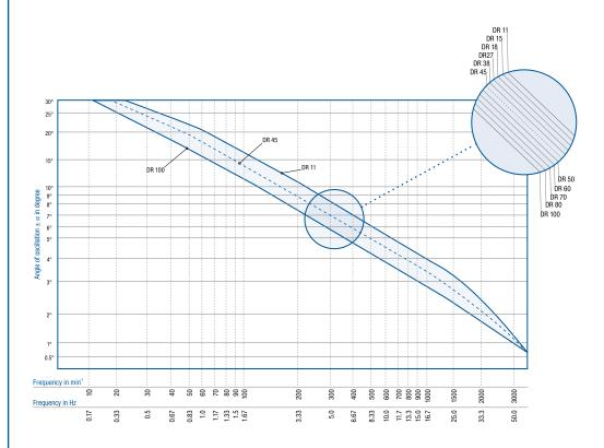
Alignment chart for determining the permissible frequencies and oscillation angles in relation to the respective rubber suspension element type (DR 11, 15, 18, etc.). The higher the frequency in min<sup>-1</sup>, the lower the oscillation
