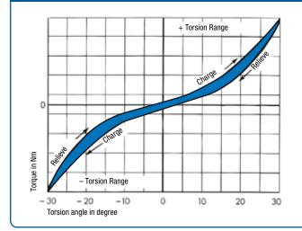
Due to the specific construction characteristics of the ROSTA rubber suspension element, pivoting the device ± results in a slightly progressive spring characteristic. The torsion angle is limited to  $\pm 30$  for most elements.
